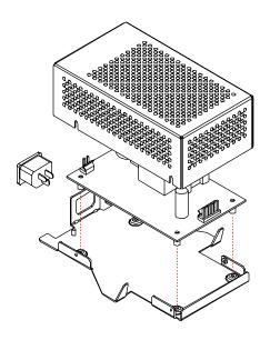
Figure 5-18. Power Supply Assembly.
